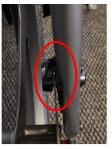
□ Unscrew the brake caliper. Take the supplied Allen key and loosen the 2 bolts.
