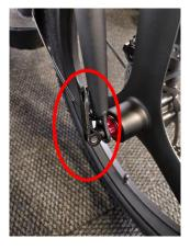
4) Turn the wheel to see if the disc is sitting nicely between the pads. If you do not hear the brake rubbing against the pads, you are safe to drive!
