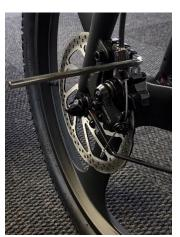
⇒ Squeeze the brake. Keep it depressed until the adjustment is complete.
